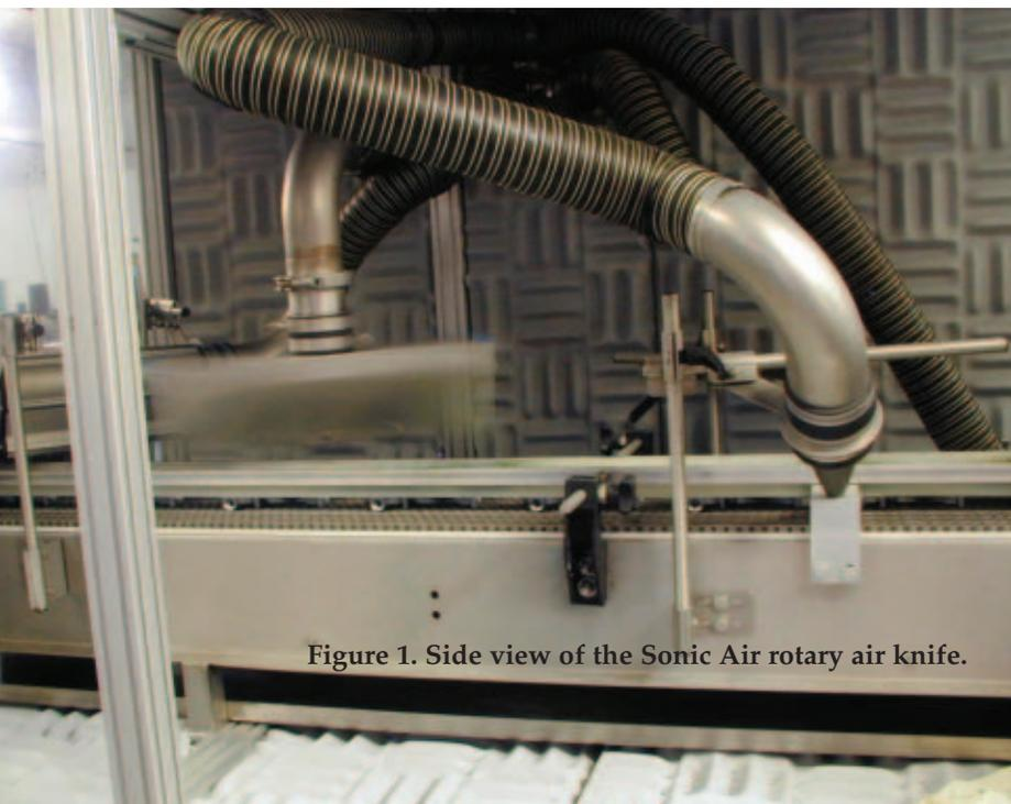
Figure 1. Side view of the Sonic Air rotary air knife.
